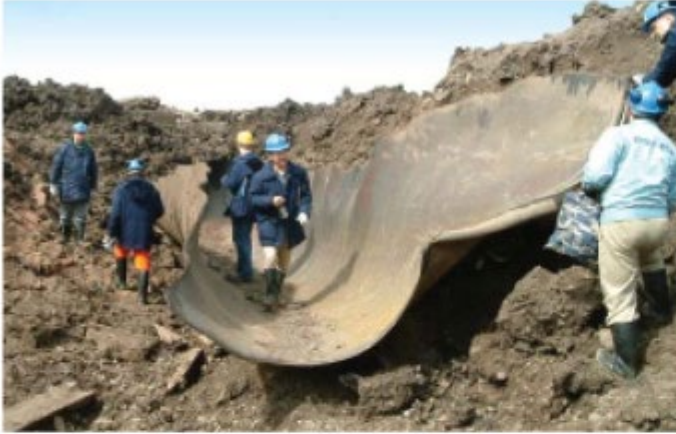
A running fracture – result of a test
