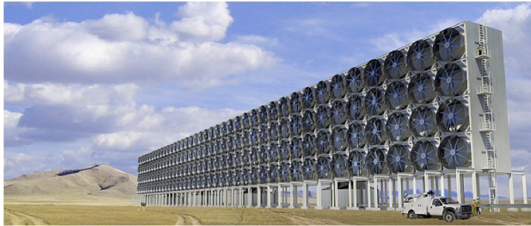
Air contractor device for direct air capture (Carbon Engineering)
